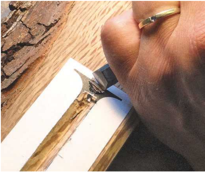
Establishing the 45° slope of the serif. Moving backwards with the chisel, achieving the correct angle
